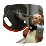
The WIVA POWER system uses an inertial sensor connected via Bluetooth to a computer and allows to determine both eccentric and concentric force during a training on BIOMECH® STUDIO Program.
